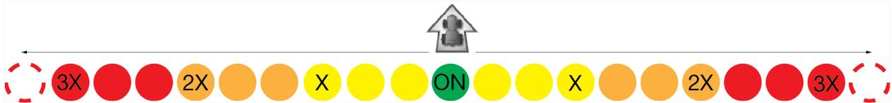
The virtual and XW-1 steering wheel lightbars differ in the number of colored lights. The XW-1 lightbar has only one light of each color which lights as the user-defined distance (**X**) is exceeded. The virtual lightbar has three lights of each color which light as one-third of the user-defined distance (**X**) is exceeded.
